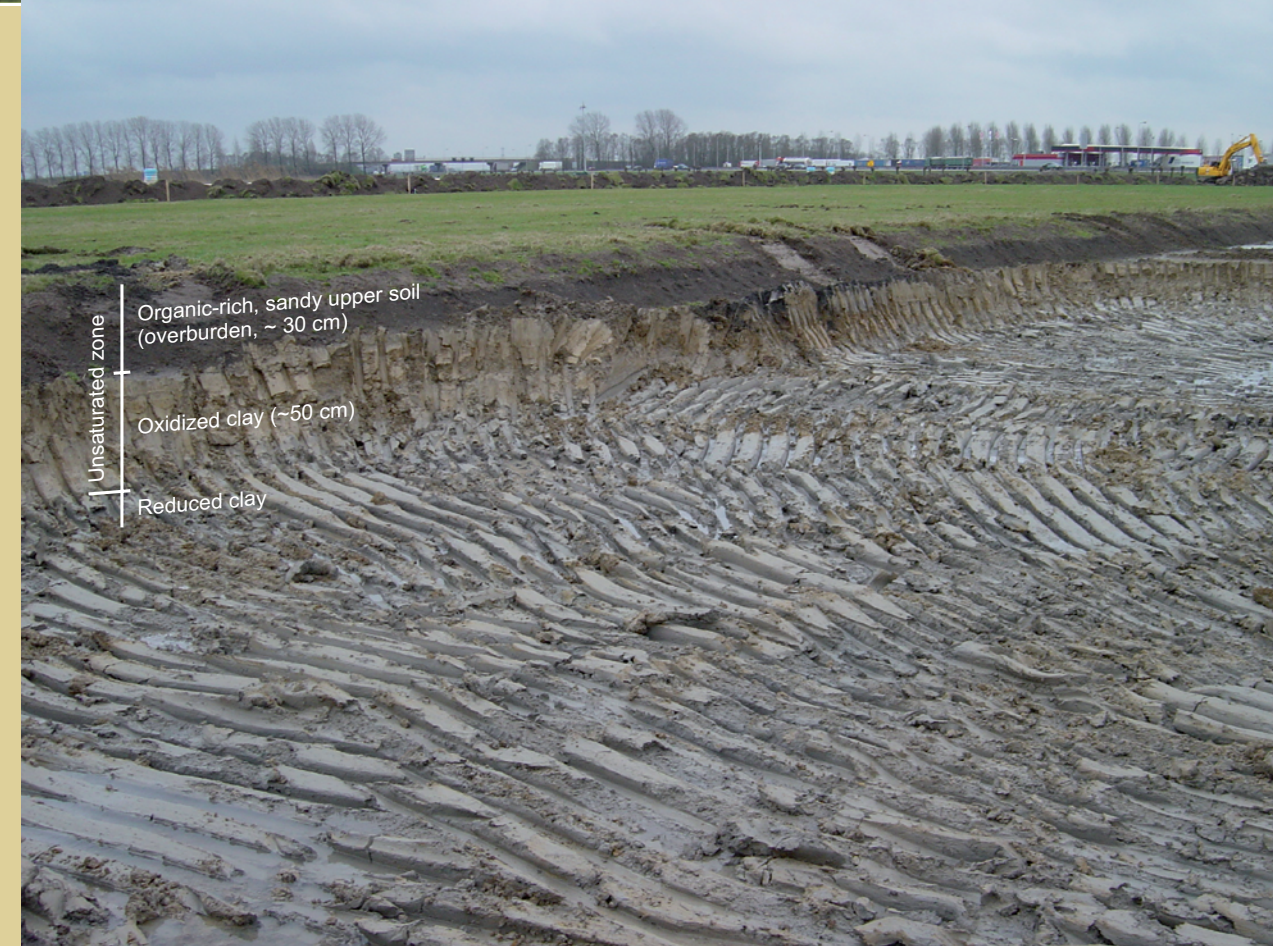
Fig. 2. Upper left panel: the extraction of clay using a backhoe. Upper right panel: the extraction depth is about 1 m (including ~30 cm of overburden); relevant lithological variation on that vertical scale is clearly visible. A caliche-horizon within the oxidised clays (not visible on this scale) presents a challenge, as it has to be removed before continuing extraction.
